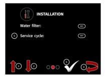
To adjust, push on 5 and on 1 or 2 until the desired number of cycles appears. **(Value up to 999000 cycles)**
