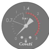
The "M1" pressure gauge indicates **the steam pressure** in the boiler.
