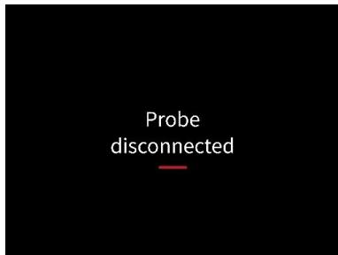
This message indicates that the electronics do not recognize the temperature sensor.
