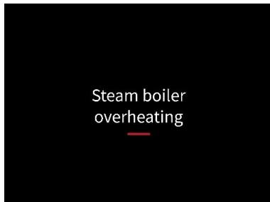
This message indicates that the electronics have detected a temperature in the boiler > at 140 °C for more than 5 seconds
